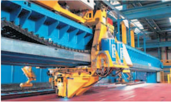
Fig. 2. Laser welding machine for panels of up to 12 m in length [2].
