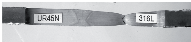
Fig. 5. Tensile test specimen. Square edge preparation weld
