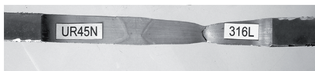
Fig. 5. Tensile test specimen. Square edge preparation weld
