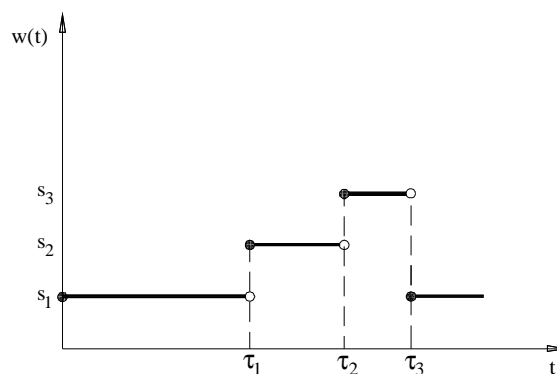
Fig. 2.. Example of realization of an engine slide bearing \{W(t): t \geq 0\} process, where: s_1 - state of full ability, s_2 - state of partial ability, s_3 - state of inability; [0, \tau_1) , [\tau_1, \tau_2) , [\tau_2, \tau_3) - state duration intervals.
