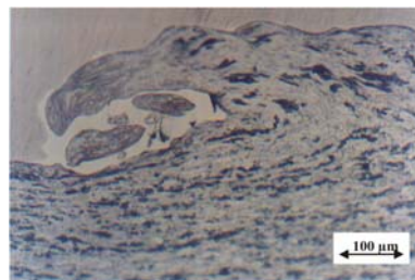
Fig 2. Microstructure of titanium – steel joint. In the area of created wave white intermetallic phase is visible [11, 12]
