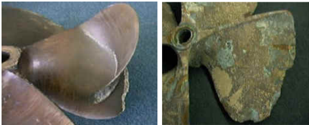
Fig.5. The examples of propeller wear and damages (źródło: http://home.xtra.co.nz/hosts/henleyspropellers/prop_damage.htm )
