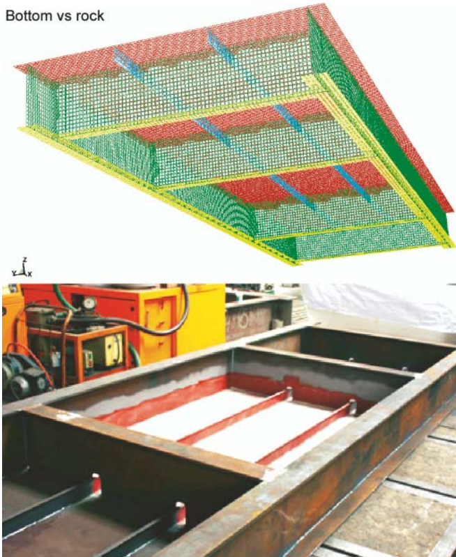
Fig. 1. Numerical model and real structure model of a fragment of ship double bottom structure
