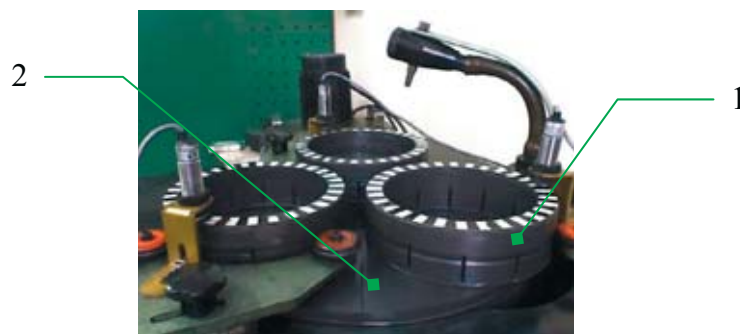
Fig. 1. Executory system of single disc lapping machine ABRALAP 380: 1- truing rings, 2-lapping tool
