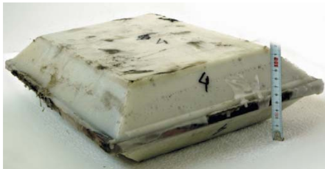
Fig. 2. The specimen covered with the polyurethane layer - concrete filler protective system
