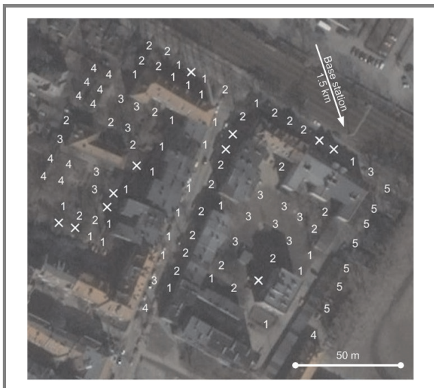
Fig. 2. WiMAX coverage hole effect: measured coverage of the WiMAX base station in 3.5 GHz band. Stable modulation profile chosen by client terminal: × – no communication; 1 – binary phase-shift key (BPSK); 2 – quaternary phase-shift key (QPSK); 3 – quadrature amplitude modulation 16 (QAM16); 4 – QAM64 1/2; 5 – QAM64 3/4.
