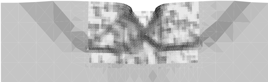
Fig. 13. Distributions of void ratio close to the footing from FE calculations with random distribution of e_o for the case '2' of Fig. 8b ( B_o = 2.5 cm): a) s/B_o = 0.2 , b) s/B_o = 0.3
