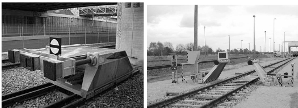
Fig. 4 Buffer stop with impact energy-absorbing buffers [4, 6]
