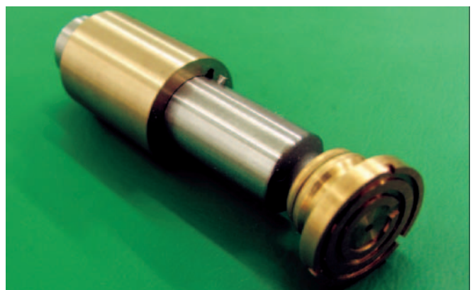
Fig. 8. Piston unit adapted to measuring the heating process
