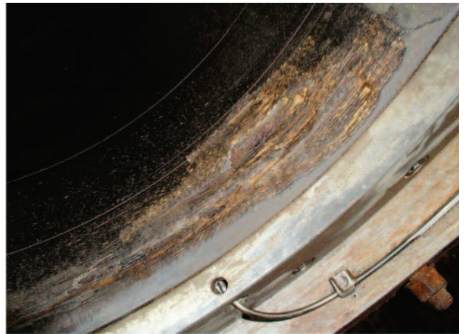
Fig. 2. Cantilever open bearing of yacht's propeller shaft
