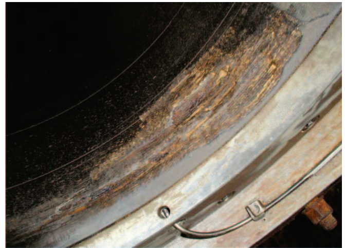
Fig. 2. Cantilever open bearing of yacht's propeller shaft
