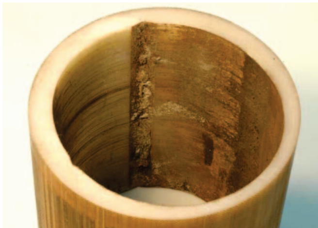
Fig. 6. An unsealed sea-water-lubricated bearing which was exposed to pollution and fouling
