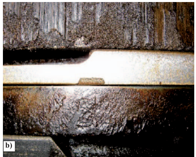
Fig. 5. Ring part of piston – the engine working on a biofuel produced on the basis of crude (not processed) palm oil.
