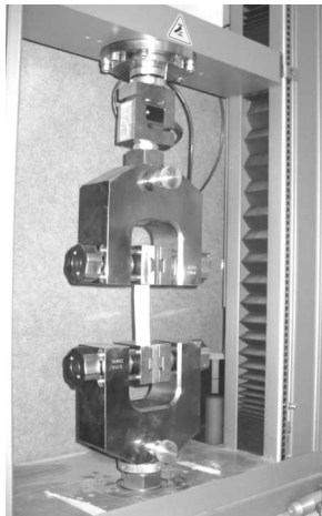
Fig. 3. One-dimensional stretching test of Dual Mesh (WL Gore) on the Zwick Roell testing machine
