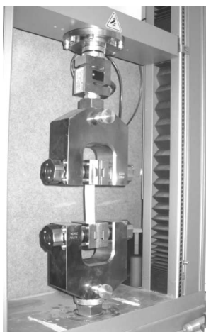
Fig. 3. One-dimensional stretching test of Dual Mesh (WL Gore) on the Zwick Roell testing machine
