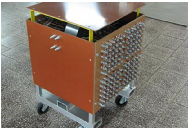
Fig. 3. External view of the RSTT. The terminal board of secondary windings is visible on the right hand side
