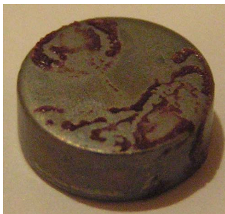
Fig. 7. Appearance of alloy surface after an exposure in Enterobacter cloacae solution
