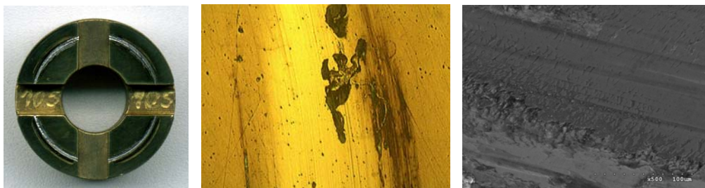
Fig. 2. Images of a TiN coated specimen after testing on PT-3 Tribometer, saline lubrication. Macroscopic image of the worn working face of the non rotating specimen (left); Optical microscopy photograph of the worn and broken coating (centre); SEM image of the border zone of the wear mark (right).
