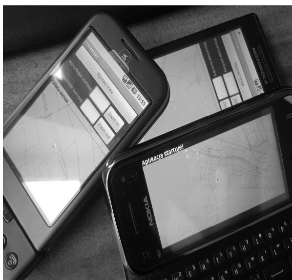
Fig. 7. Prototype application on three different smartphones: Nokia n97 mini (Symbian+JavaME), Motorola MileStone and T-Mobile G1 (both Android).
