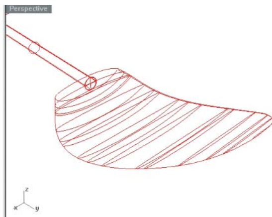
Fig. 3. Design of the model hydrofoil
