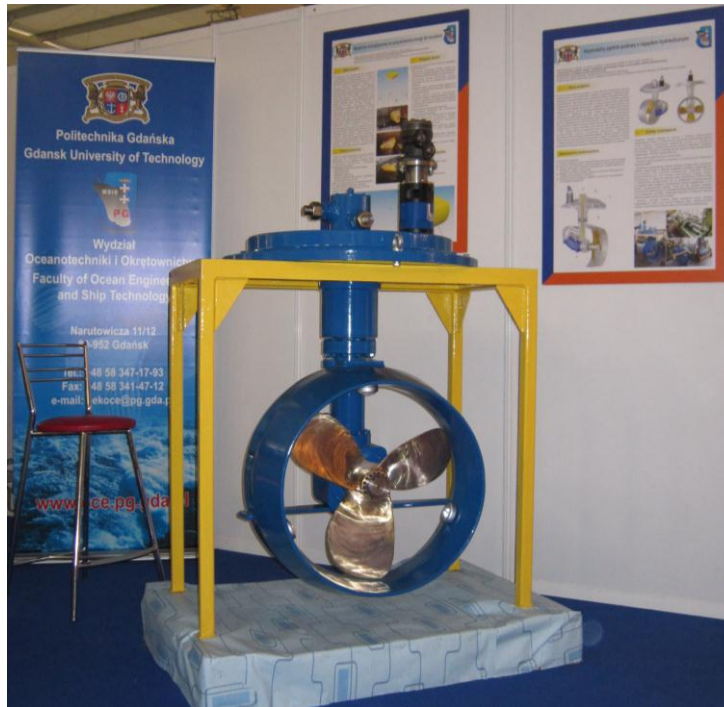
Fig. 6. Photography of the azimuth podded thruster presented on the 16th International Maritime Exhibition BALTEXPO – 2011 in Gdansk
