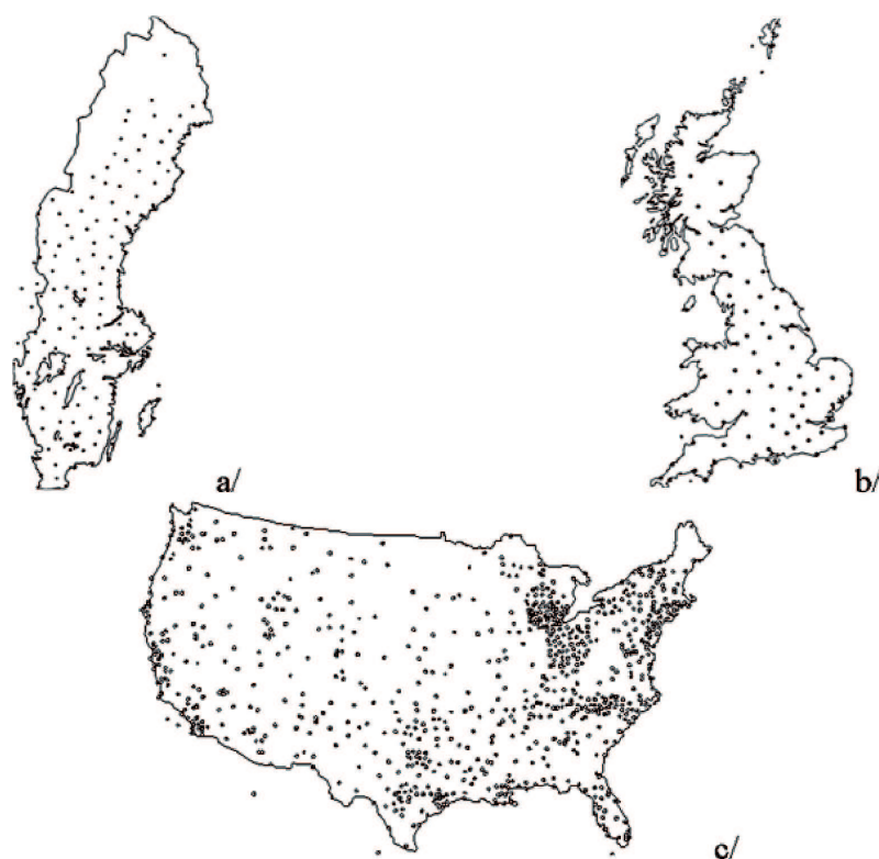
Fig. 1. Architecture of chosen active geodetic networks: a/ SWEPOS – Sweden, b/ OS-AGN – Great Britain, c/ CORS – USA
