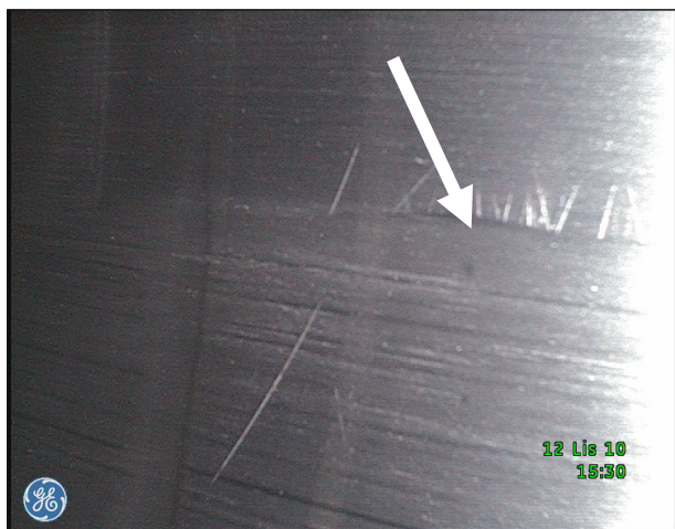
a) cylinder bearing surface - friction traces originated from the piston leading part
