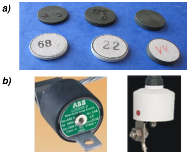
Fig. 7. Selected varistor measured specimens: a) disc-shaped ZnO structures after being fired (top row) and with metalized contacts (bottom row), left 280 V, middle 440 V, right 660V, b) surge arresters with these varistors
