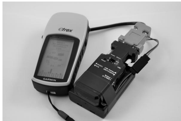
Fig. 2. DGPS measurement unit.
