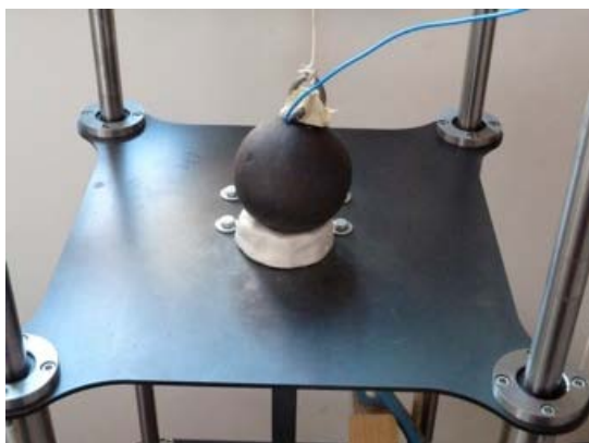
Fig. 4: Moving platform with the steel sphere and clay pad
