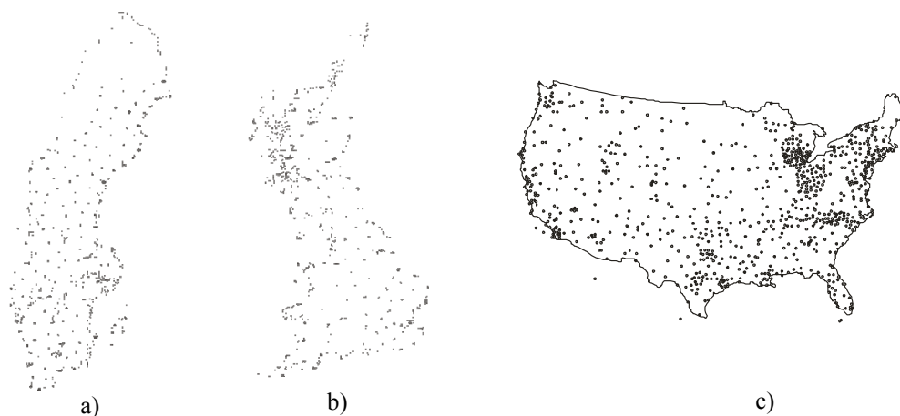
Fig. 1. Architecture of chosen active geodetic networks: a) SWEPOS — Sweden; b) OS-AGN — Great Britain; c) CORS — USA [own study]
