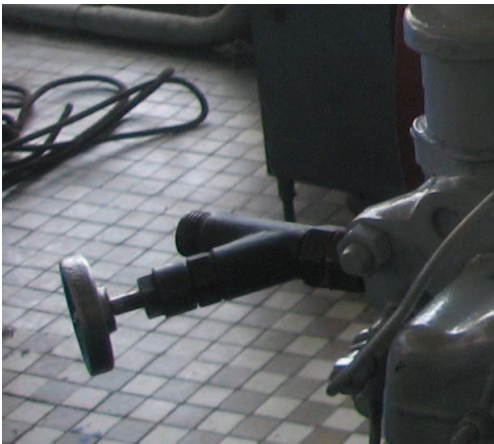
Fig. 2 Indicator valve installed in a place of holder of ignition paper (a) an electronic indicator PREMETS XL on a laboratory stand (b)
