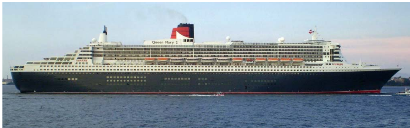
Fig. 1. The passenger ship Queen Mary 2 with visible life boats placed on ship sides [7]
