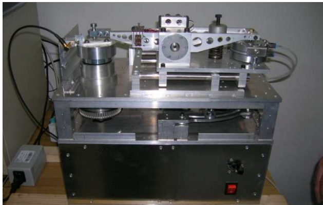
Fig. 3. Prototype of the device with an eccentric oscillation inducer
