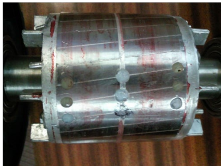
Figure 3: Broken rotor bars and central end ring.
