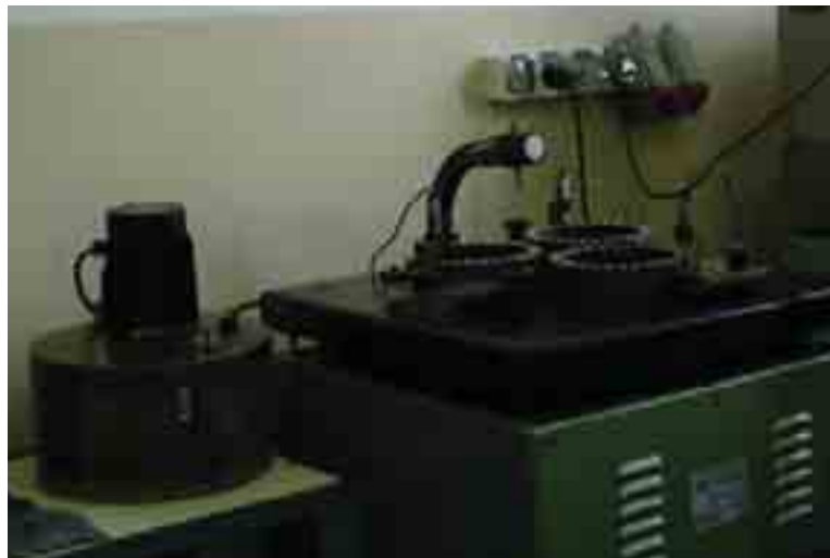
Fig. 3. One-plate lapping machine ABRALAP 380
