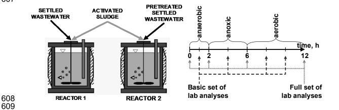
Figure 2. Feed source, operating sequence, and analyses for experiments with two parallel batch reactors (parameters measured in the basic and full sets are described in the text)
