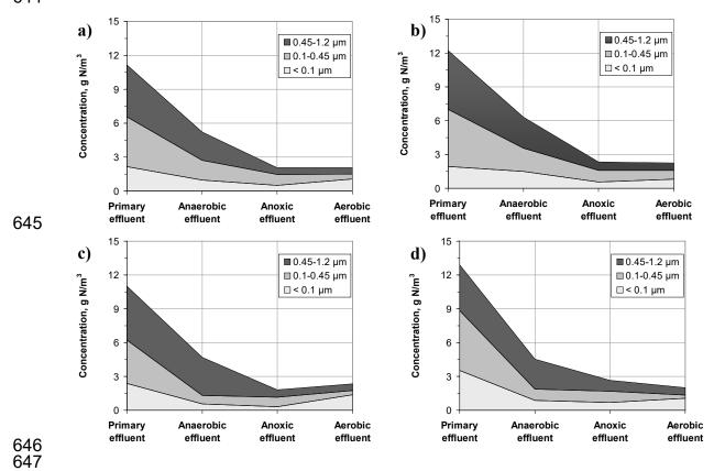
Figure 6. Average concentration profiles of DON and CON in the full-scale bioreactors (fall and spring study sessions) at the Gdansk WWTP (a-b) and the Gdynia WWTP (c-d)
