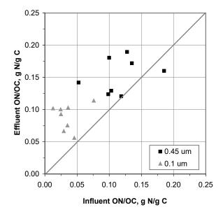
Figure 4. Effluent DON/DOC vs. influent DON/DOC in the 8 studied BNR WWTPs based on filtration through 0.45  $\mu m$  and 0.1  $\mu m$  pore-size filters
