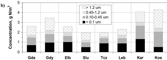
Figure 3. Primary and secondary effluent ON fractions in the 8 studied BNR WWTPs
