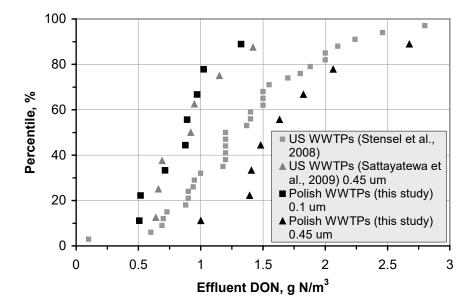
Figure 5. Probability distributions of secondary effluent DON concentrations
