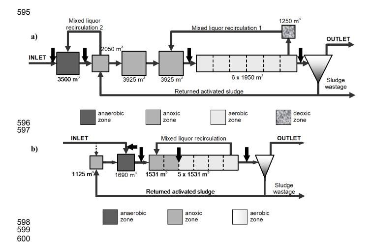
Figure 1. Schematic of BNR system bioreactor compartments: (a) Gdansk MUCT process, (b) Gdynia JHB process (black arrows show sampling locations)
