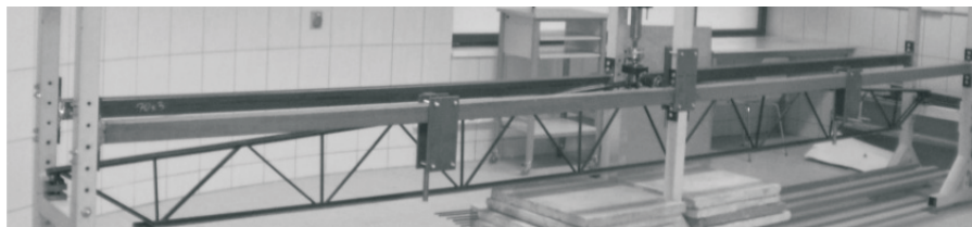
Figure 2 Experimental set-up of truss with elastic braces
