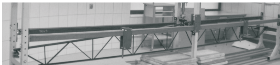
Figure 2 Experimental set-up of truss with elastic braces
