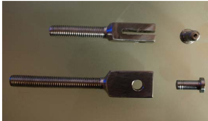
Fig. 3. Clamps fixing the specimens
