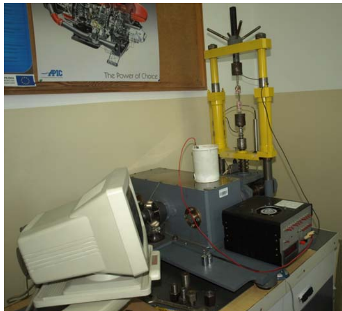
Fig. 2. Equipment for slow strain rate tests
