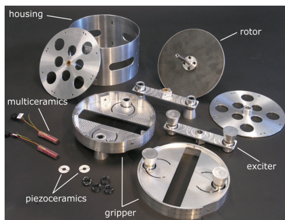
Fig. 12. Disassembled prototype hybrid piezoelectric motor [6]
