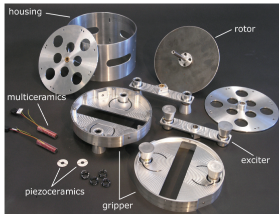
Fig. 12. Disassembled prototype hybrid piezoelectric motor [6]
