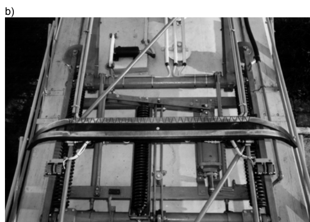
Fig. 1. Currently operating contact line diagnostic system DST, where: a) view of measuring car; b) measuring current collector with sectional contact tip [5]
