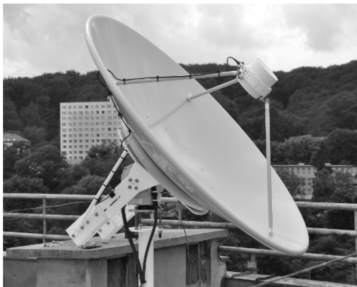
Fig.1. Antenna of the 1.5m HRPT/MetOp ground station.
