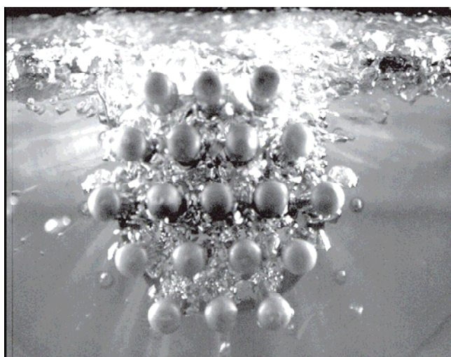
Fig. 10. Visualization of intensifying steam bubble effect for water boiling process on a porous coated tube bundle; s/D = 1.7 , at atmospheric pressure ( p = 100.5 \text{ kPa} ) and heat flux q = 30.25 \text{ kW/m}^2
