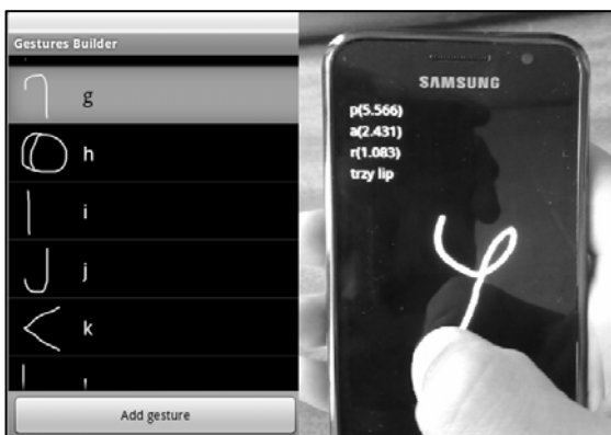
Figure 2. Gesture keyboard for the blind (Kamiński et al. 2011).
