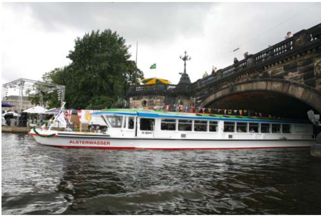
Fig. 1. The Alsterwasser ship launched in 2008 in Hamburg, driven with a 100 kW electric motor supplied by two 48 kW fuel cells, may take a hundred passengers on deck ( http://www.zemships.eu )
