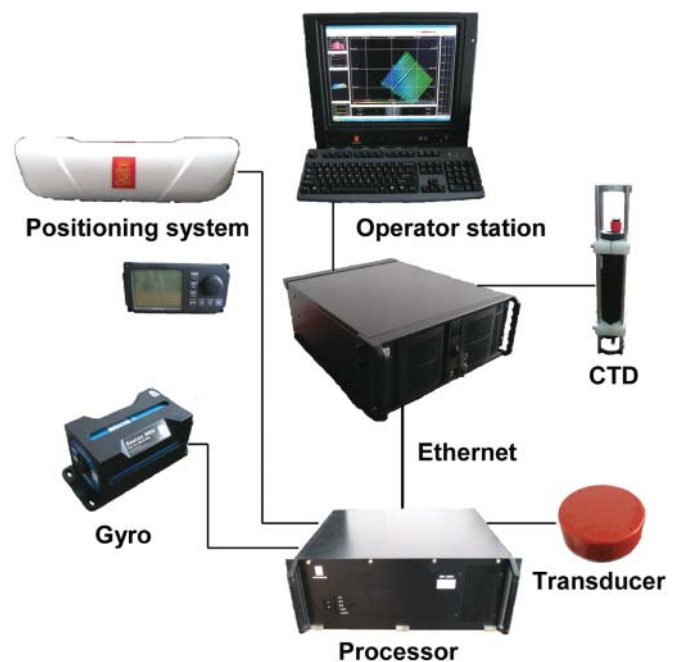
Fig. 1. The overview of multibeam sonar system structure
