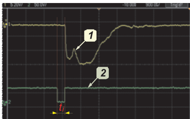
Fig. 11. Determination of the advance or delay time t_i of the Langmuir probe versus the TDC signal
