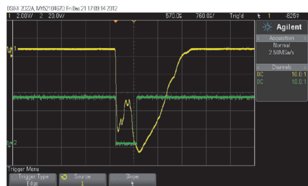
Fig. 7. The Langmuir probe signals (above) and the TDC pulses (below) measured for the Farryman D10 Diesel engine at greater time resolution
