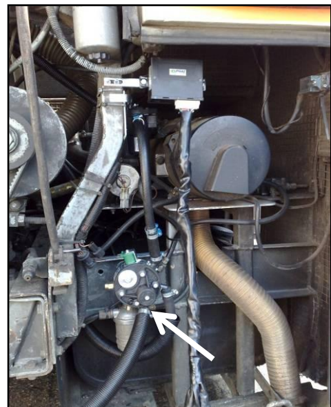
Fig. 3.4. The example of the evaporator montage in bus
