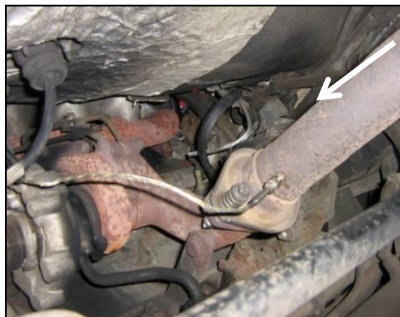
Fig. 3.6. The example of exhaust thermometer montage
