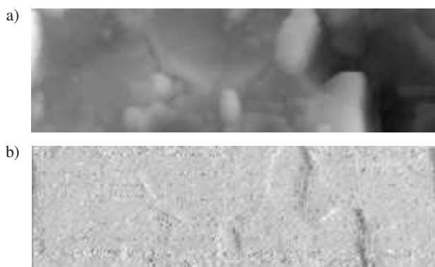
Fig. 7. Topography of graphene observed in tapping-mode made by dedicated software (a) and image of the second harmonic component (b)
