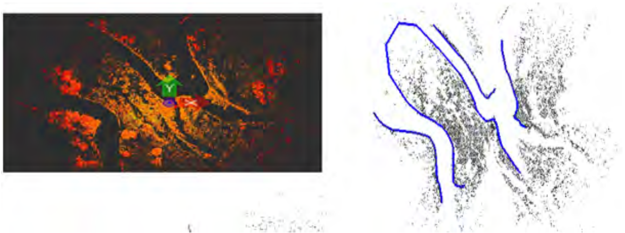
Fig. 3. Point cloud from TLS after the initial filtration (Own work)
