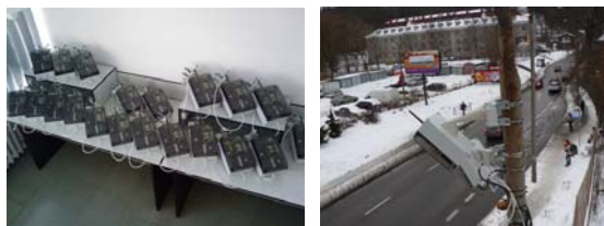
Fig. 5. The pictures of the assembled sensor nodes and one of them installed on the street lamp – pole (FPGA prototype #2)
