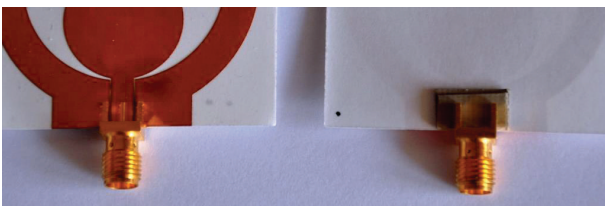
FIGURE 4: Photographs of the SMA connector and the brick under the feeding line.
