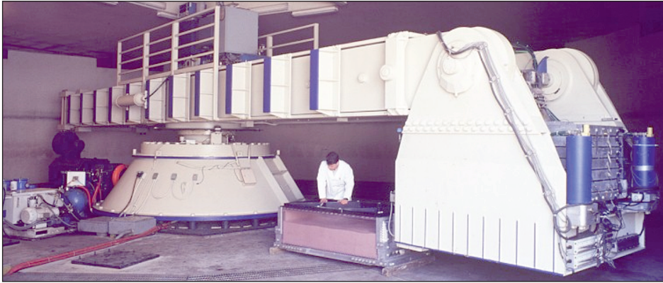
Fig. 1. Geotechnical beam centrifuge in Davis, University of California
