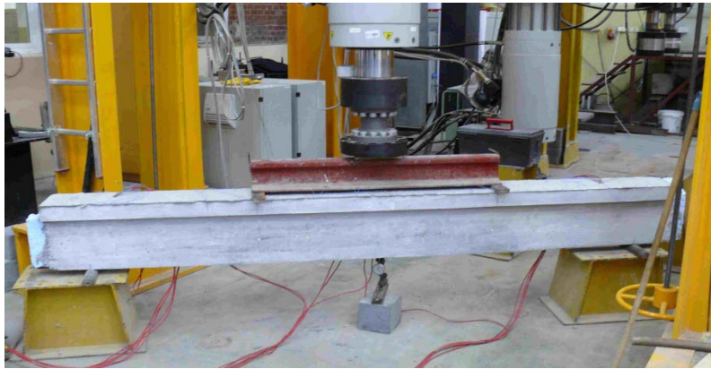
Fig. 5. The beam at the setup
